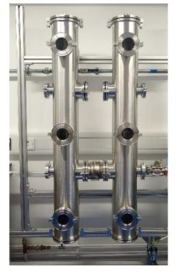
Novel absorber test rig under construction at UoW
